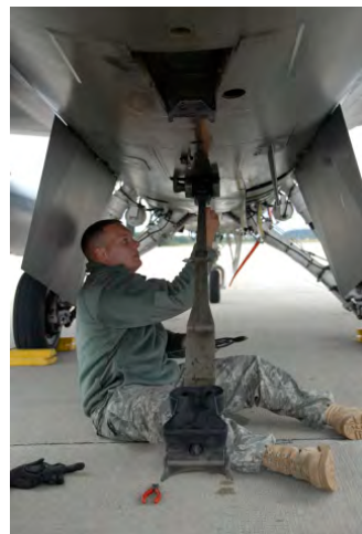
Staff Sgt. Jordan Jensen, a crew chief with the 115th Fighter Wing in Madison, Wis., resets the tail hook on an F-16 Fighting Falcon that is used to "hook" the Barrier Arresting Kit 12 cable installed at the end of each runway, a system designed to stop an aircraft
