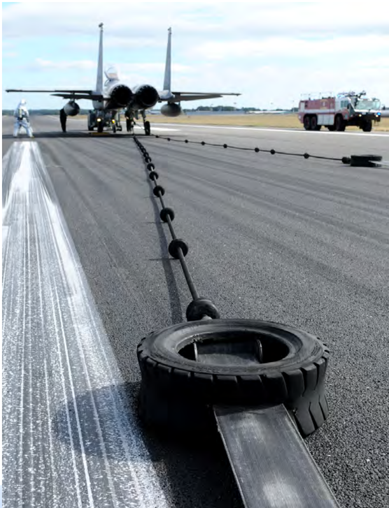
RAF MILDENHALL, England – Emergency crews tend to an F-15 from the 48th Fighter Wing, RAF Lakenheath, after it was stopped by arresting gear during an exercise Sept. 22. The gear must be checked annually, so the fighter engaged it while taxiing at about 90 knots. (U.S. Air Force photo/Staff Sgt. Austin M. May)
